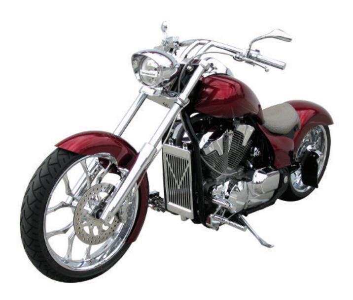
The following front ends will fit custom applications on Metric motorcycles. They were originally designed for use on Harley Davidson Custom bikes but metric custom builders can utilize the following front ends on any triple tree applications that will accept 41mm front forks. We list the Harley applications to simplify the installation of other components ie HD wheel applications, HD brake rotors and calipers, triple trees, axles and spacers etc.
