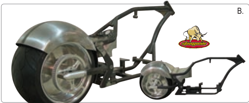
Frames include: Oil Tank, Swingarm w/ Hidden Axle Adjusters, Flush-Mount Side Plates, Axle Housing And Internal Forkstop Plate
